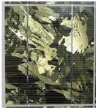
Figure I.11 : Cellule photovoltaïque poly-cristalline
