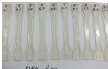
Figure 9. Tensile specimens in Polyester resin
