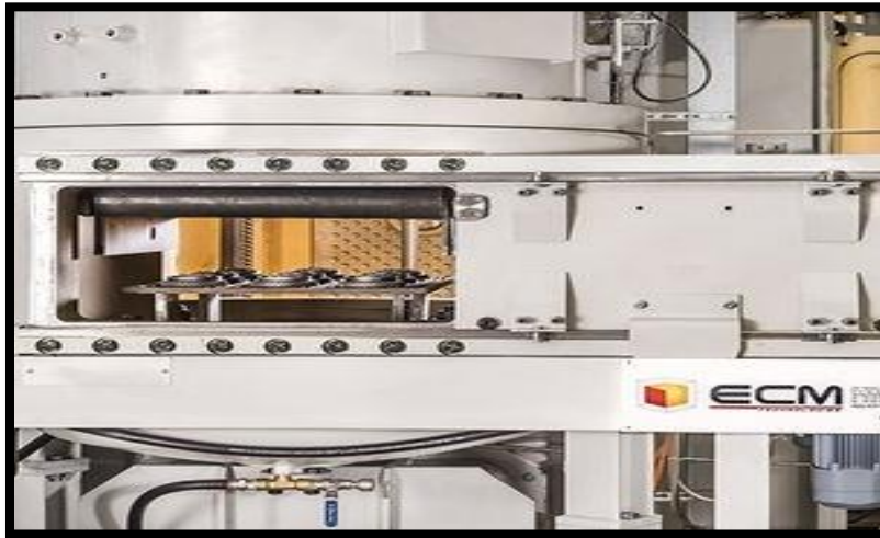
Figure III.2. Four automatique de cémentation.
