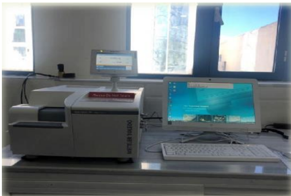
Figure II.8: TGA instrument (TGA/ DSC 3+ 1600°, METTLER TOLEDO).
